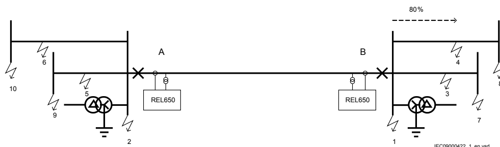
Figure 27: Fault points for phase overcurrent setting calculations
